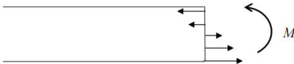
Fig.2: Stress distribution through the thickness of a plate and resultant bending moment
